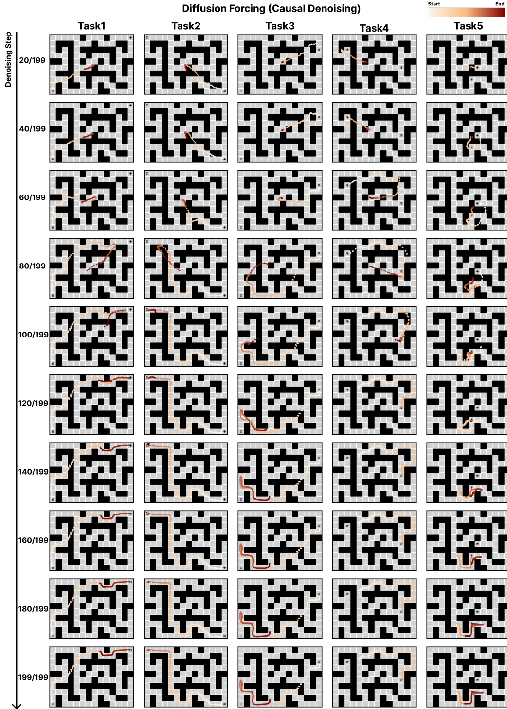
Figure 35: Denoising visualization for Diffusion Forcing. We visualize predicted clean trajectories \hat{x}_0 at selected denoising steps. Causal denoising can resolve early prefixes before later horizon regions are sufficiently revised.
