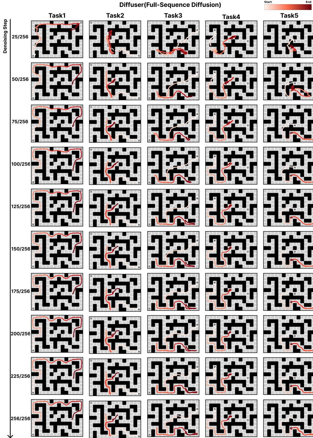
Figure 34: Denoising visualization for Diffuser. We visualize predicted clean trajectories \hat{x}_0 at selected denoising steps. Full-sequence diffusion can commit to an early incorrect plan.
