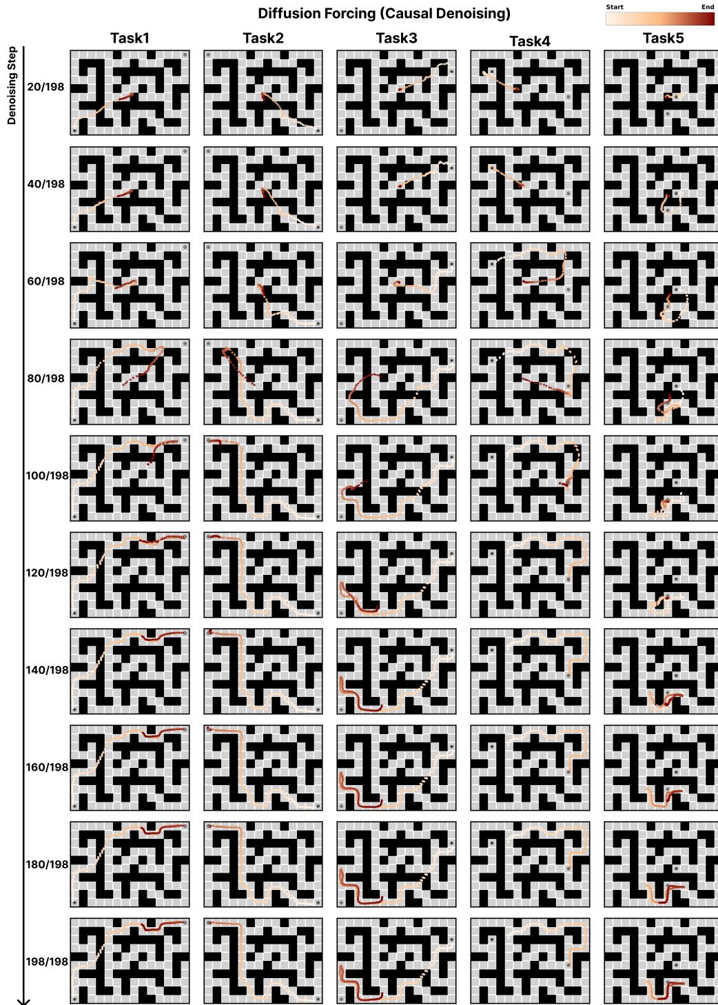
Figure 26: Denoising visualization for Diffusion Forcing. We visualize predicted clean trajectories \hat{x}_0 at selected denoising steps. Causal denoising can resolve early prefixes before later horizon regions are sufficiently revised.
